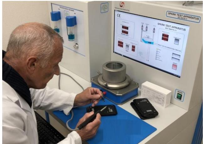
*All modifications are tested in the explosive atmosphere of the spark-test apparatus for intrinsically safe circuits*
